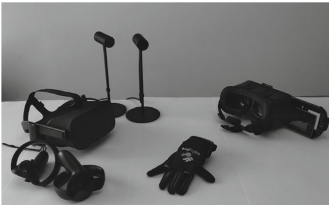
Fig. 12.1 Different devices for VR. On the left, the Oculus Rift and its Constellation; On the right, the Gear VR with a mobile phone in it; In the middle, a Glove controller
