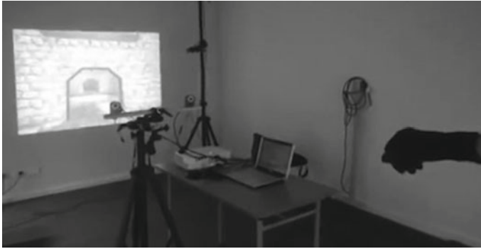
Fig. 12.2 Preliminar setting of a CAVE with only one wall projection and infrared cameras for tracking glove movements
