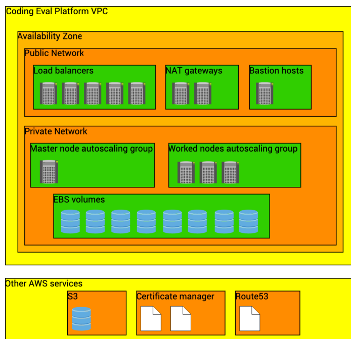
Figure 2: Graphic overview of the provisioned infrastructure used to deploy the platform.
