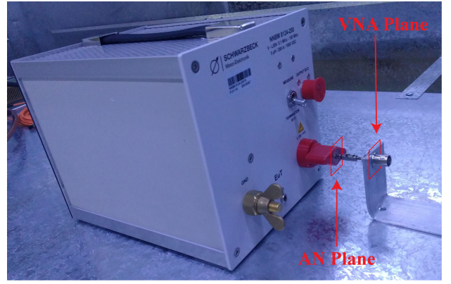
Fig. 6: Artificial Network with the VNA calibration plane and the shifted reference plane for the impedance definition.
