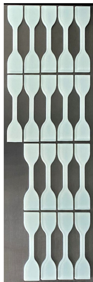
Fig. 4. Picture of the set of the 18 specimens after finishing the printing process.
