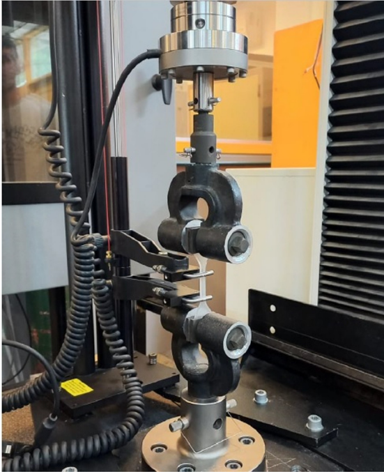
Fig. 5. Instron 3382 performing the tensile tests on a printed sample.
