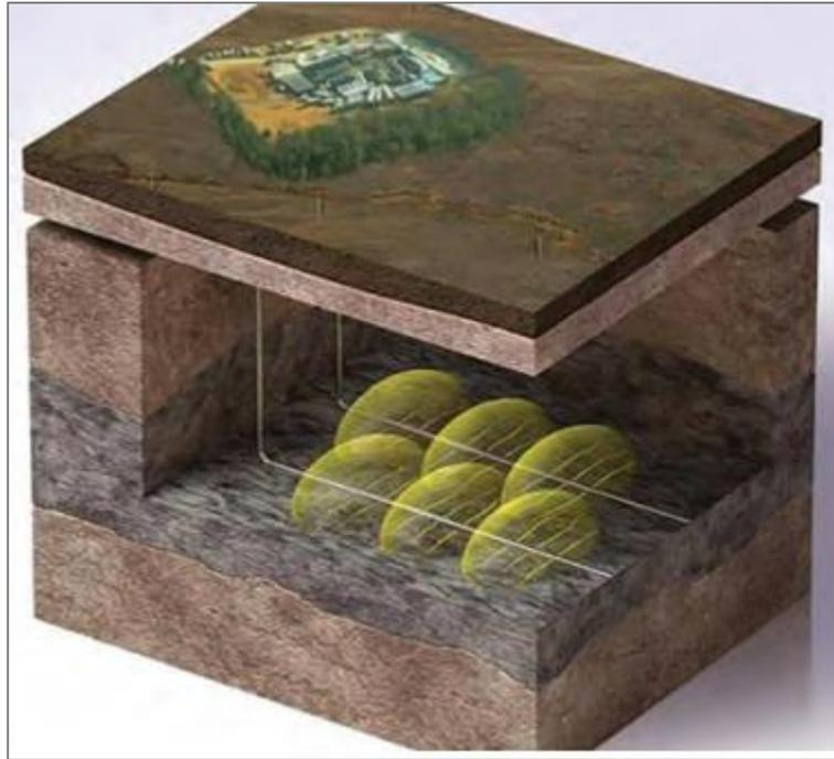
Figura 20. Zipper fractures.
