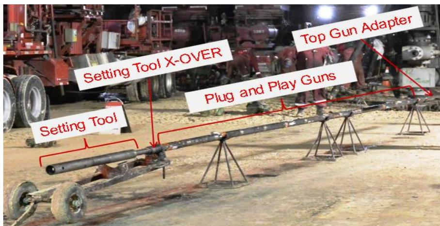
Figura 12. Plug & Perf guns and setting tool. (Halliburton, 2020).
