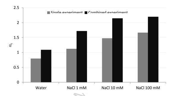
Fig. 6: Collision efficiency factor  $(\alpha_c)$  for  $TiO_2$  in the single experiment and pseudo-collision efficiency factor for  $TiO_2$  in the combined experiment.
