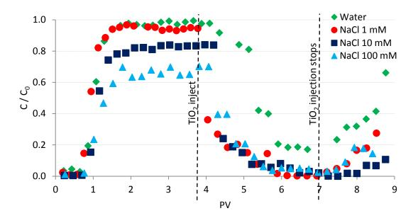
Fig. 4: Breakthrough curves for bacteria, measured by qPCR between 4 and 9 PV, in co-transport of bacteria and TiO<sub>2</sub>.
