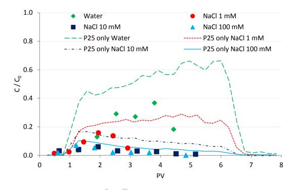
Fig. 5: Breakthrough curves for titanium measured by spectrophotometry at 410 nm after digestion and addition of  $H_2O_2$  in co-transport of bacteria and  $TiO_2$ . Breakthrough curves for  $TiO_2$  only for comparison.
