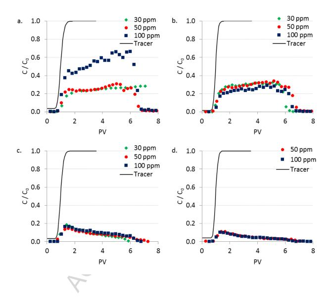
Fig. 2: Breakthrough curves for  $TiO_2$  in sand columns suspended in different media: a. Ultrapure water (resistivity 18 M $\Omega$ .cm); b. 1 mM NaCl; c. 10 mM NaCl; d. 100 mM NaCl. pH=5.2-5.8.
