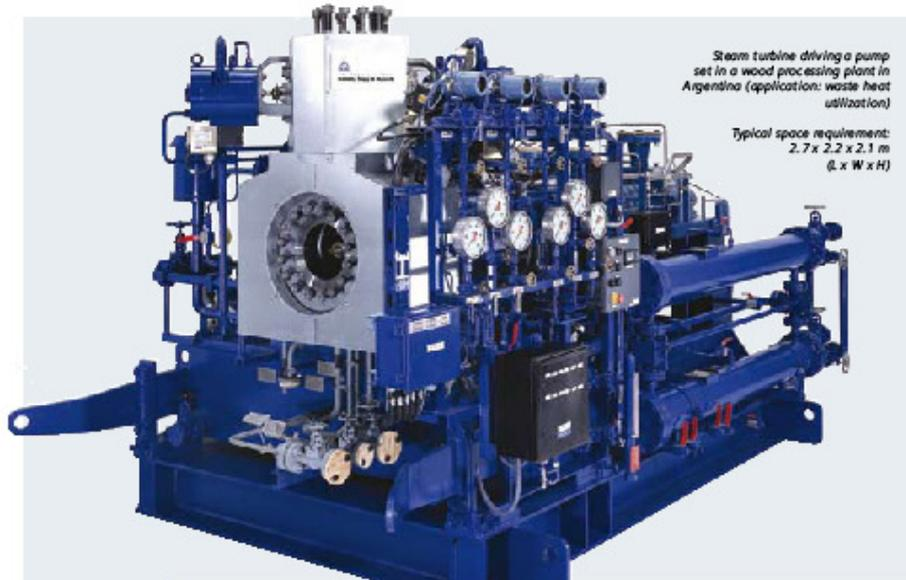
Steam turbine driving a pump set in a wood processing plant in Argentina (application: waste heat utilization)
