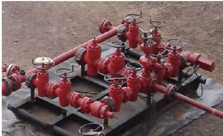
*Fig.20.1– Choke Manifold*
