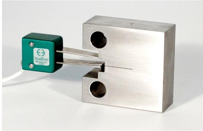
**Figura 21:** Clip gage colocada sobre una probeta compacta (Epsilon Tech-<https://www.epsilontech.com/products/fracture-mechanics-cod-gage-model-3541/>).
