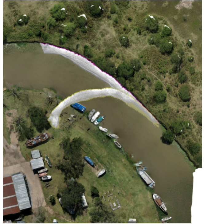
Figure 10: Map obtained with Cartographer (magenta trace using IMU data and yellow trace without using IMU data) overlaid on aerial mosaic.
