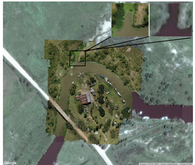
Figure 11: Mosaic composed of aerial photographs with Google Maps image in the background for resolution comparison.
