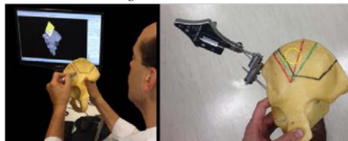
Figure 1 – A Plastic Pelvic bone showing color lines that depict each planning and execution method. Black line: 2D planning and freehand. Red line: 3D planning and freehand. Green line: 3D planning and navigation guidance. The yellow circle shows the estimated location of the tumor.
