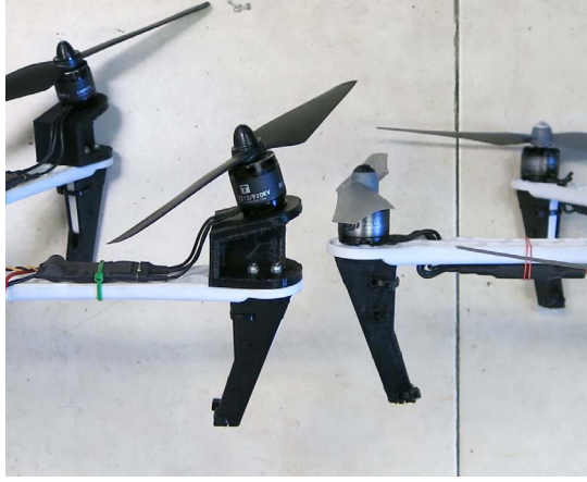
Figure 4. Detail of rotor mounting configuration. Left: tilted-motor hexacopter . Right: standard hexacopter.
