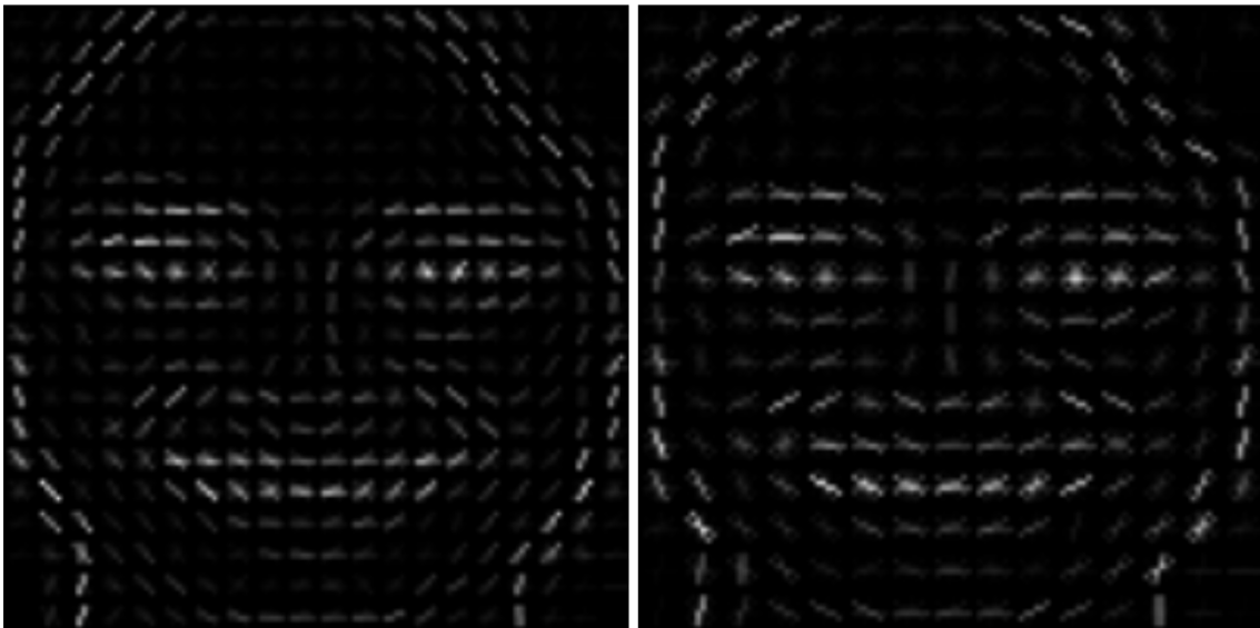
Figure 13: Superimposed image of applying HOG descriptor with cells of 6x6 and 8x8 respectively
