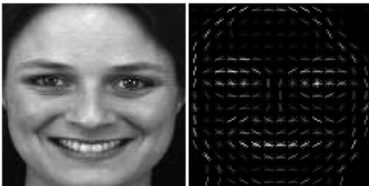
Figure 5: Original image (left) and the result of applying the HOG method (right).
