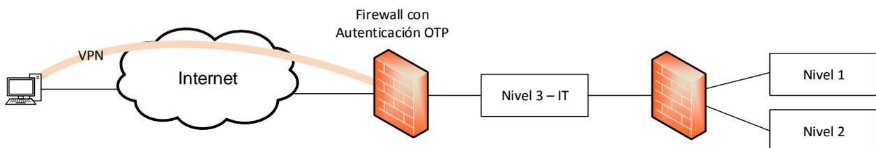
FIGURA 14: ESQUEMA ACI. INTERNET A NIVEL 1 O NIVEL 2
