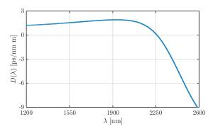
Fig. 1. Proposed waveguide: (Top) mode distribution and (bottom) dispersion  $D(\lambda)$  of a silicon nanowire lying over a silicon-dioxide substrate. White lines separate different materials , and yellow lines indicate the 2D-decoration layer.
