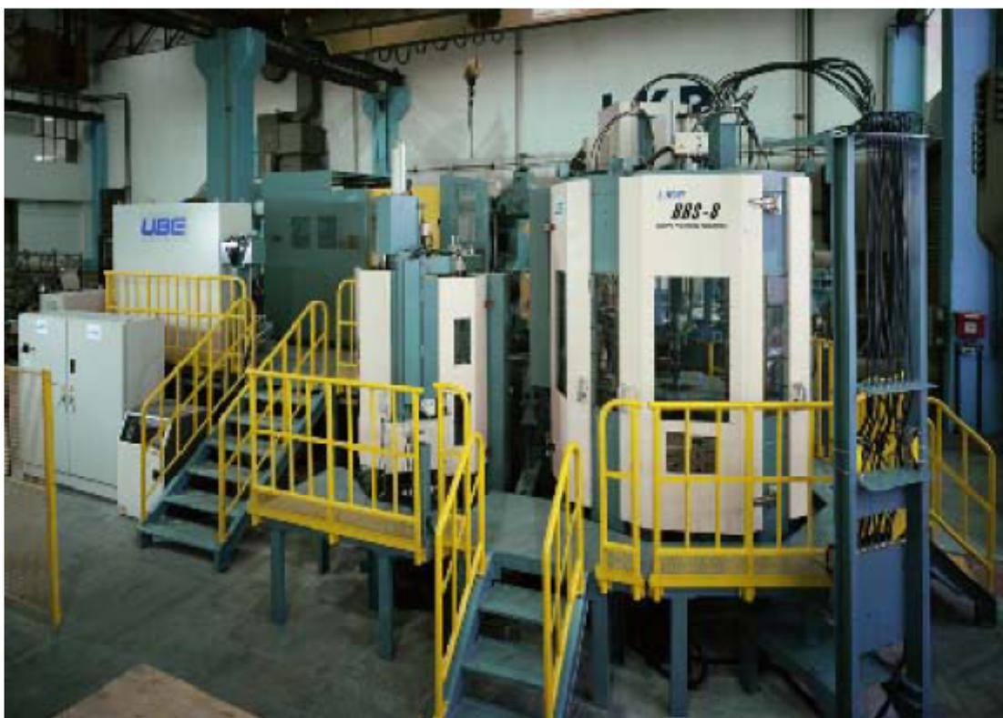
**Figura 7.14.** Máquina de New Rheocasting UBE HVSC PL-800 NRC
