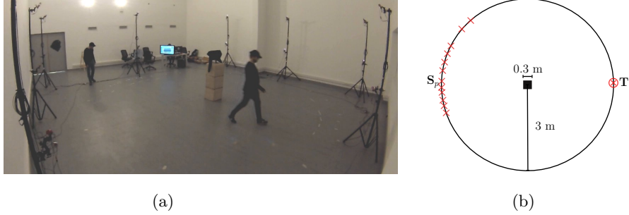
Figure 2: Experimental setting. (a) Snapshot of the experiment. (b) Schematic representation of starting points ( \mathbf{S}_p ) and final target ( \mathbf{T} ) for the recorded trajectories.
