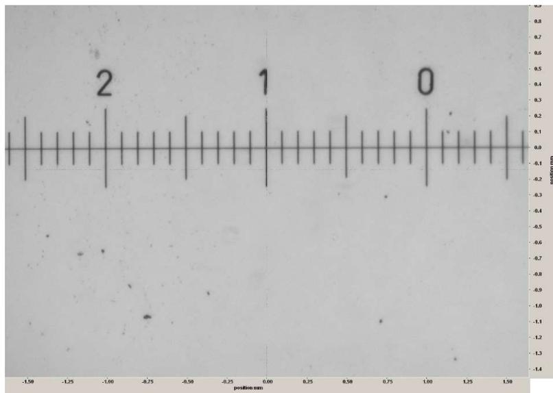
Figure 4.3: Taken Image of the scaling plate.
