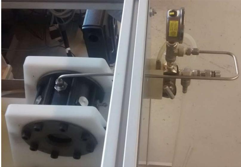
Figure E 4: Optical chamber, pressure valves and gauge – New connection.
